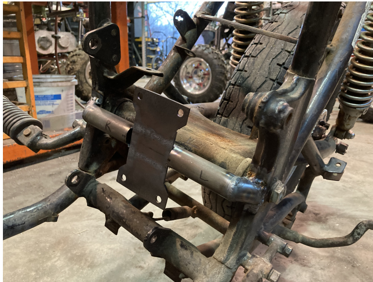
Figure 12: Custom Motor Mount on the Frame
