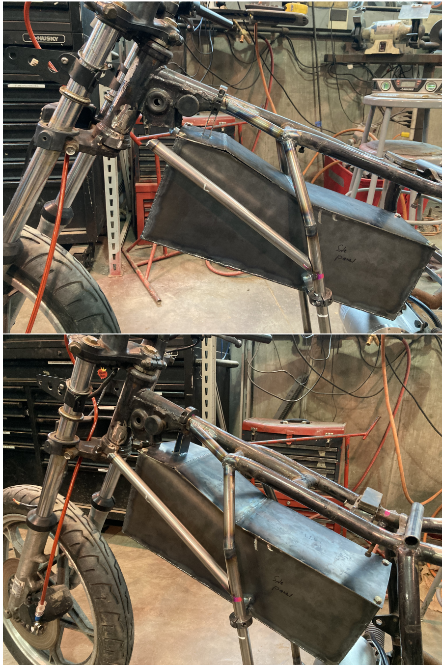
Figure 21: Battery Enclosure fixed to Frame Only using Shaft Collars
