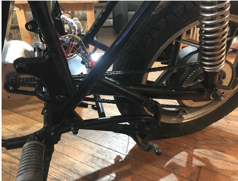
Figure 14: Final Chain Drive Configuration
