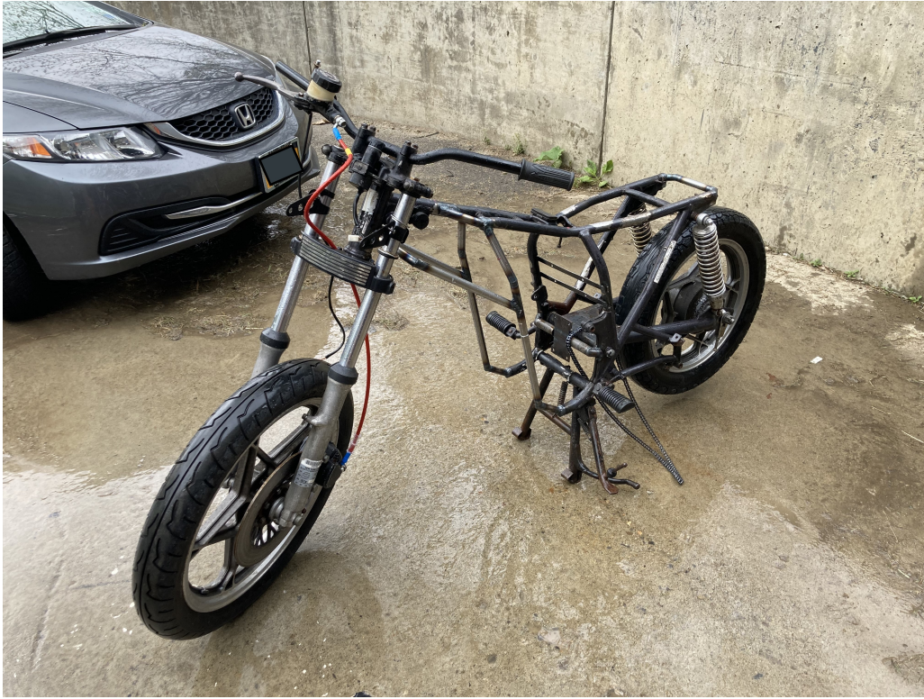
Figure 29: Bare Frame after Power-washing
