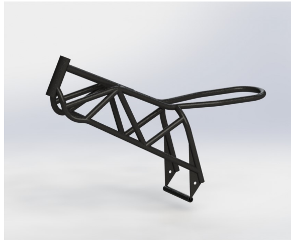
Figure 27: Trellis Frame Design v3 (part of minimalist concept using rear monoshock)
