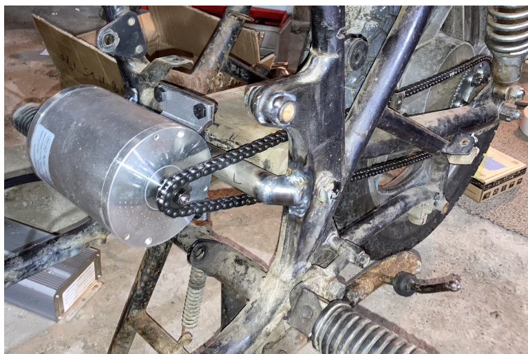
Figure 13: Custom Motor Mount & Motor on the Frame
