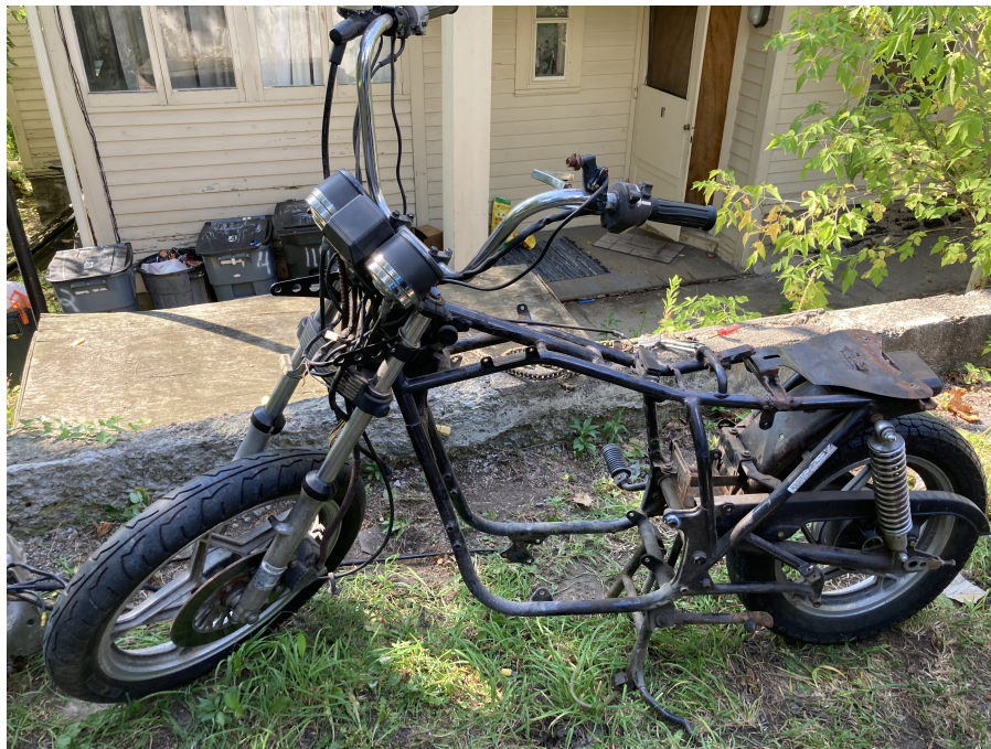
Figure 3: Removing exhaust, fuel tank and wiring
