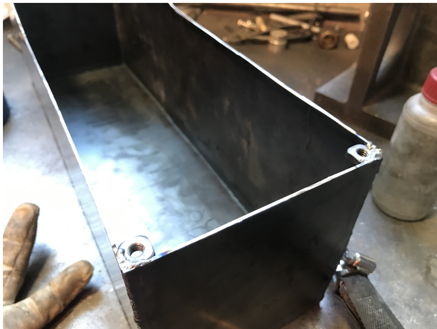
Figure 20: Weld Nuts Used in Battery Enclosure for Lid Fixture
