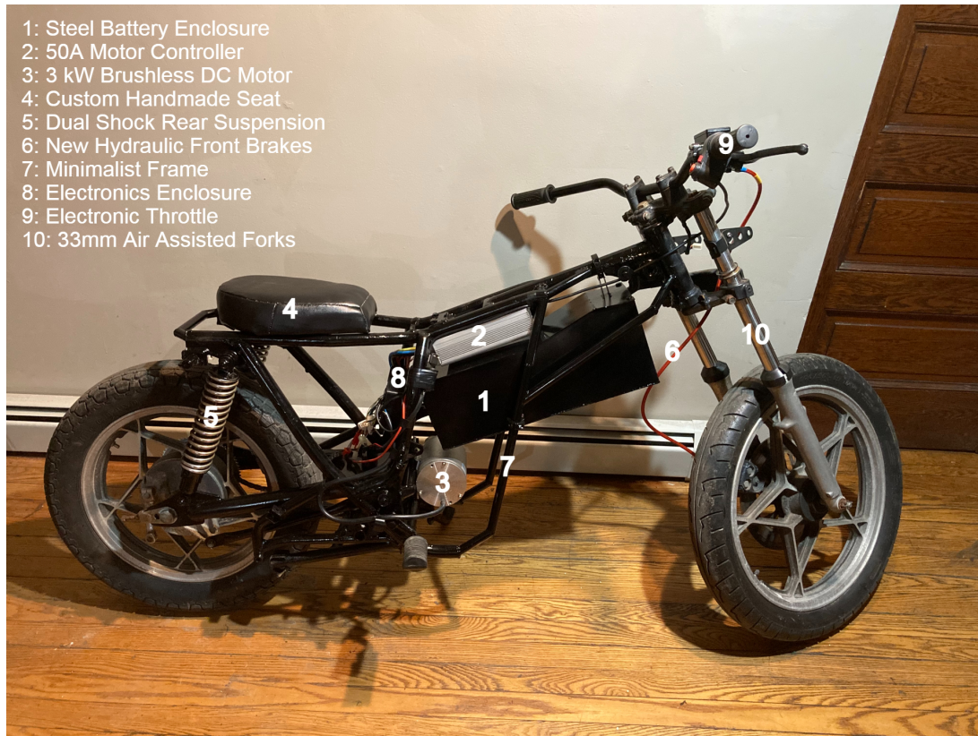
Figure 1: Completed Electric Motorcycle (Labelled)
